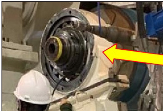
Large size bearings on paper machine rolls that need high-viscosity grease for proper lubrication.
